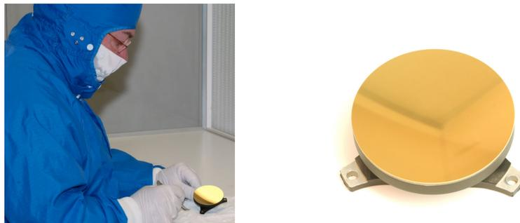
**Fig. 3. Inspection of the parabolic M1 mirror. The mirror is made of 6061-T6 Aluminum, Alumiplate<sup>®</sup>, diamond turned, and gold coated. The M1 mirror support is a so called "wine-glass" type.**
